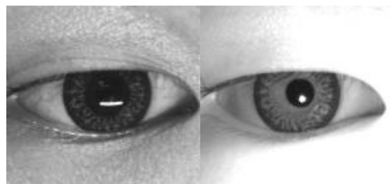
Fig. 1. (right) Image captured under near infrared and (left) image captured under visible light.
